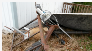
Figure 1. Pieces of the salvaged satellite dish system before moving. The welded steel post, bracket and supports are shown with the aluminum feedstock and the 10-ft dish itself, and are in good condition given their age.
