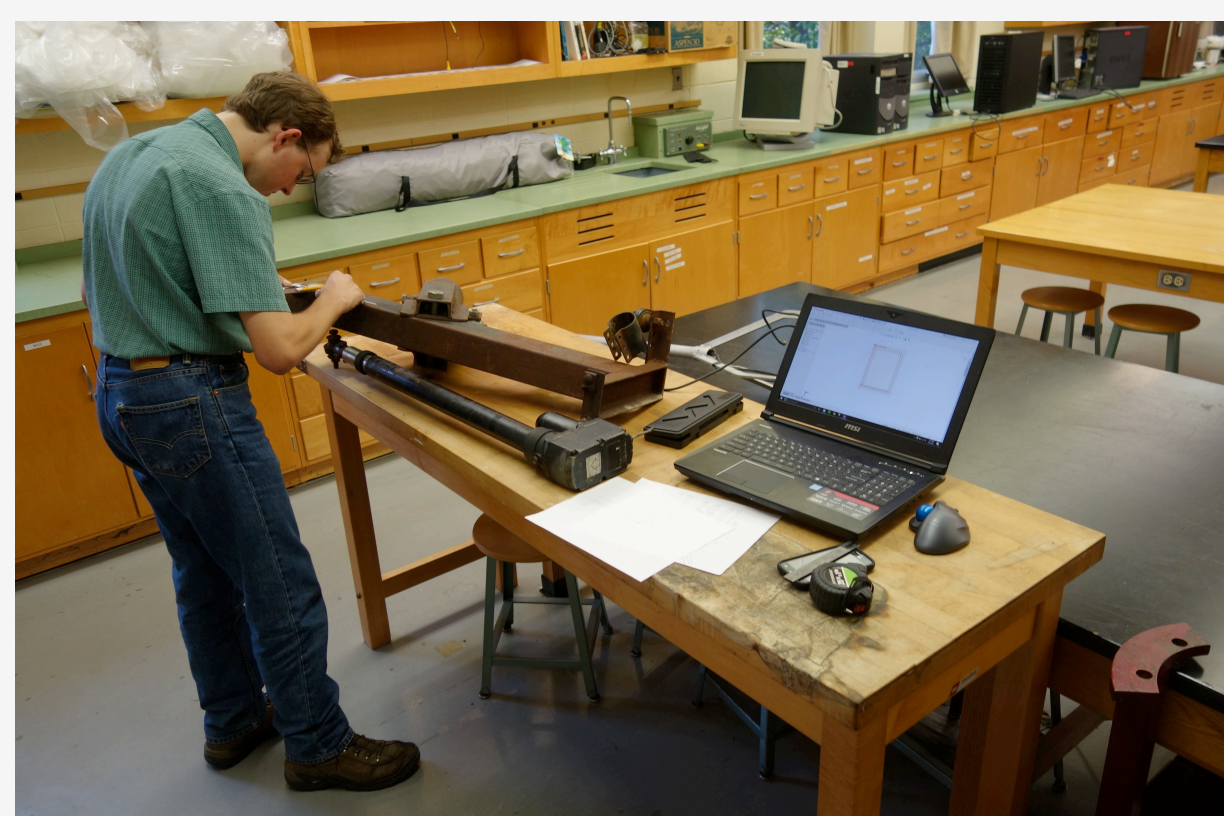
Figure 6. P. Wilkerson transferring measurements of the east-west slew actuator piston and mounting bracket into a SolidWorks Computer Aided Design software model to evaluate the telescope support structure's range of motion and to track needed replacement hardware, including new galvanized nuts, bolts, and bearings.
