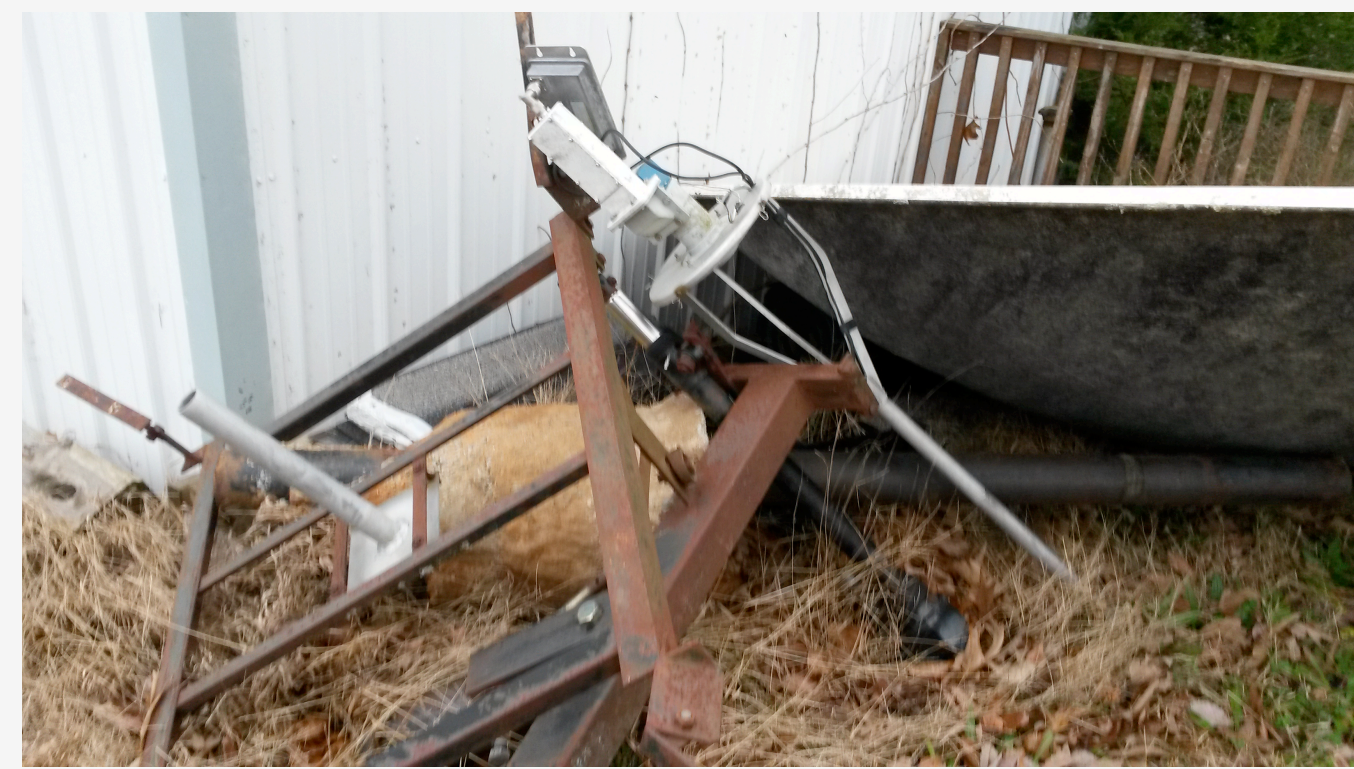
Figure 1. Pieces of the salvaged satellite dish system before moving. The welded steel post, bracket and supports are shown with the aluminum feedstock and the 10-ft dish itself, and are in good condition given their age.
