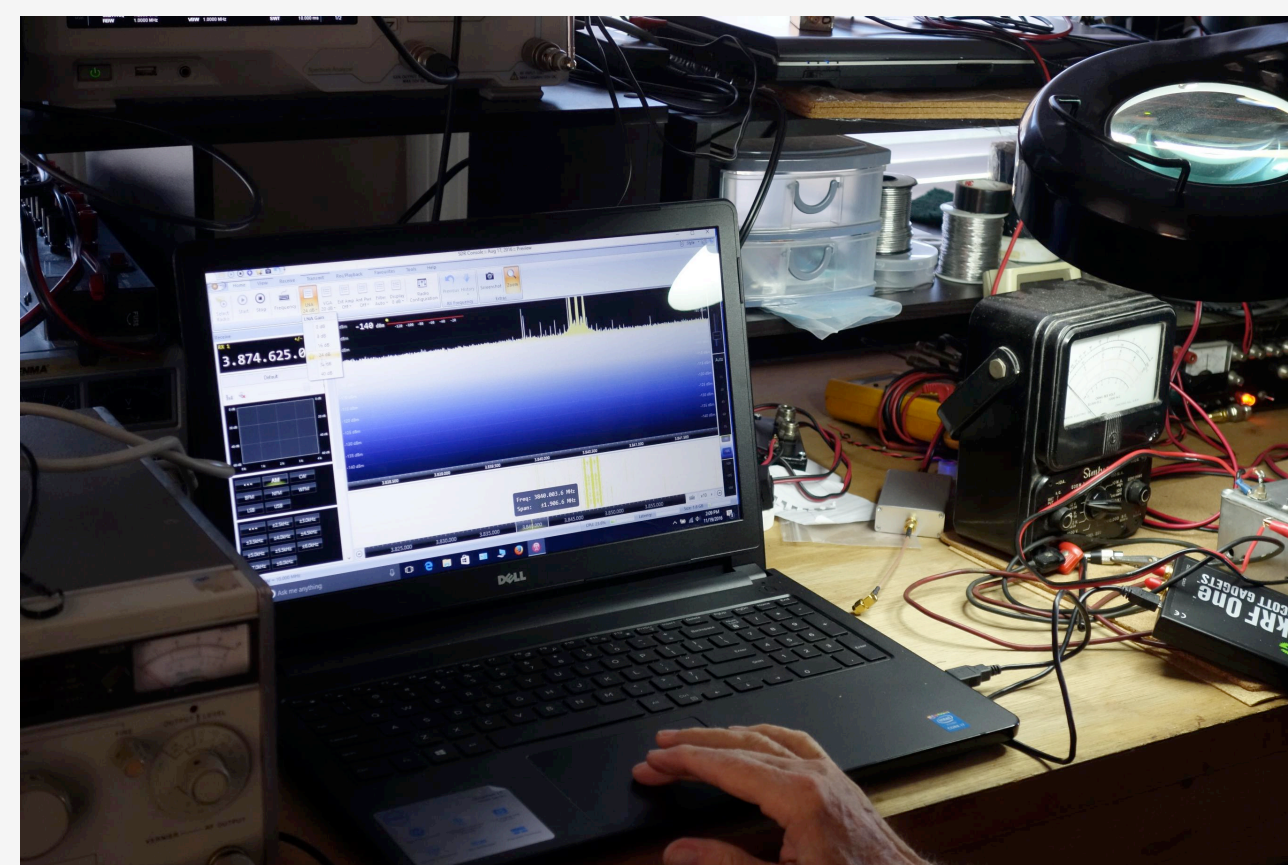
Figure 4. H. Cantrell's testing workbench with laptop showing received power vs. frequency and time in "waterfall" display from radio telescope feed.
