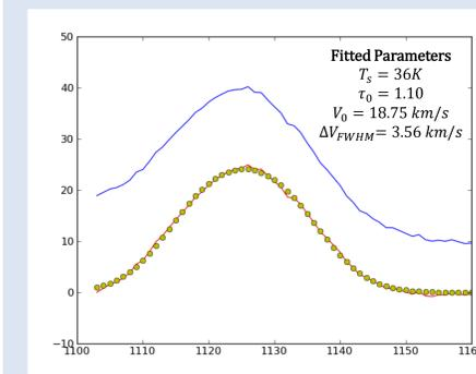
**Figure 5:** Modeling the feature. The x-axis is the velocity channel. The y-axis is the brightness temperature in kelvins. The blue line represents the observed line profile. The red line is the data with the background emission removed. The yellow dots are the resulting fit, which is not consistent with a large optical depth.
