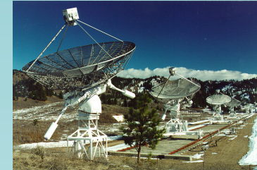
The Dominion Radio Astrophysical Observatory Synthesis Telescope, an interferometer array made up of seven connected radio dishes in British Columbia, which was used to observe the Canadian Galactic Plane Survey data used in the analysis.
