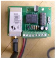
IEEE802.11b/g Wi-Fi protocol is being used for wireless communication. The switch generates a random number and compares that to a stochastic value generated by the prediction algorithm. Based on this comparison, the control signal to the compressor is either interrupted or allowed to function as normal. Research into existing cycling programs and other means of energy conservation is being conducted under this project as well.
