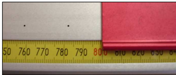
Figure 8: Verifying the calibration using a position at 0.800m
