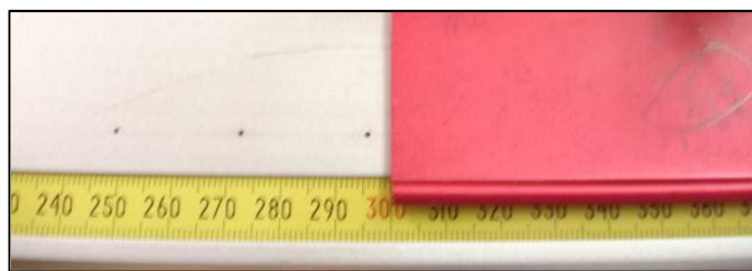
Figure 6: First calibration point at 0.300 m
